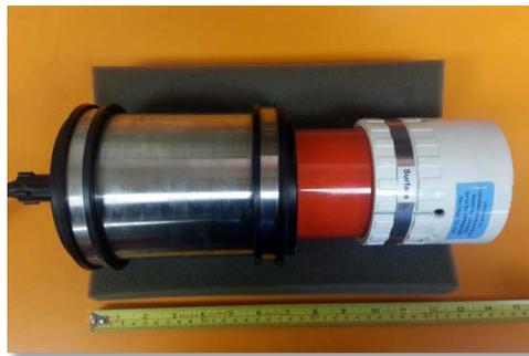
Figure 6: Underwater modem.
